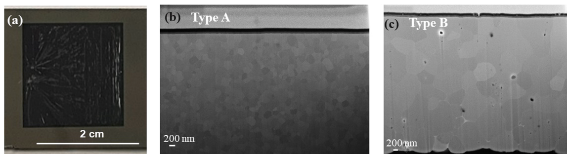
Fig. 9. (a) Photographic image of 2 \times 2 cm 2 size chip of 100 \mu m hole size sample of Type A sample after ignition and reaction completion. (b) and (c) are cross section images prepared with FIB cut of the reacted 10 \mu m hole size sample of Type A and 10 \mu m hole size sample of Type B to demonstrate the variation in the grain size after the reaction in Al/Ni multilayers.
