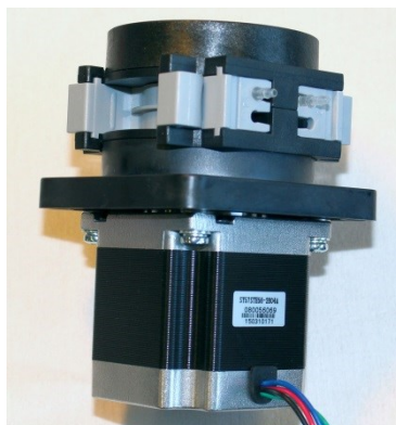
Figure 3.3 Selected stepper motor driven peristaltic pump
