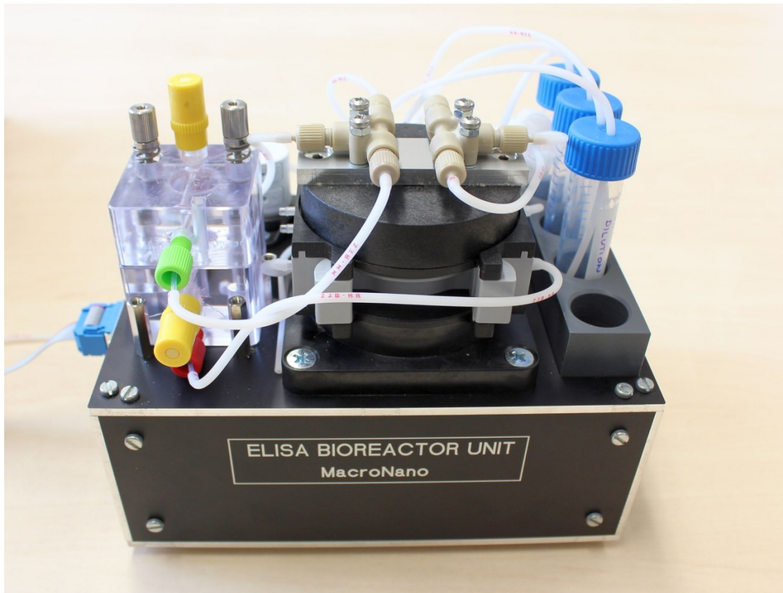
Figure 4.7 The culture unit prototype
