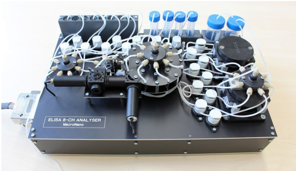
Figure 3.39 The automated flow-through ELISA module prototype
