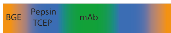
Figure 17. Sandwich-like plug setup in the second dimension. The capillary was filled with BGE, then a large plug of pepsin/TCEP mixture was injected and positioned via pressure in the valve loop with some overlap. The mAb peak was transferred from the first dimension in a heart-cut fashion.
