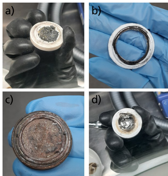
Figure 96. Post-mortem images of a \text{Na}/\text{NiCl}_2 -cell with a \text{TiO}_2 doped \text{Na}-\beta'' -alumina electrolyte. a) Cathode-side of the electrolyte b) Teflon-sealing of the cathode side c) metal inlay of the cathode side d) anode side of the electrolyte.
