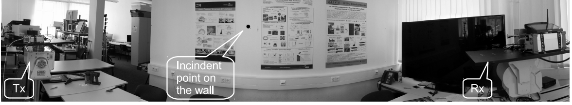
Figure 5.4: Measurement set-up for cluster-level fading investigations at 60 GHz.
