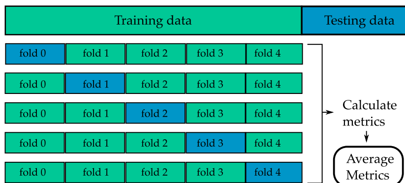
Figure 8.6.: Visualization of k -fold cross-validation with k = 5 on training data (adopted from (Sklearn Documentation 2021)). Five iterations with different combinations of training and testing folds are performed, the achieved metrics are collected and finally averaged. For each iteration different portions from the training data is used for actual training, and one portion from the training data is used for validation, i.e. testing the hyperparameter performance. The actual testing data is not considered for cross-validation.
