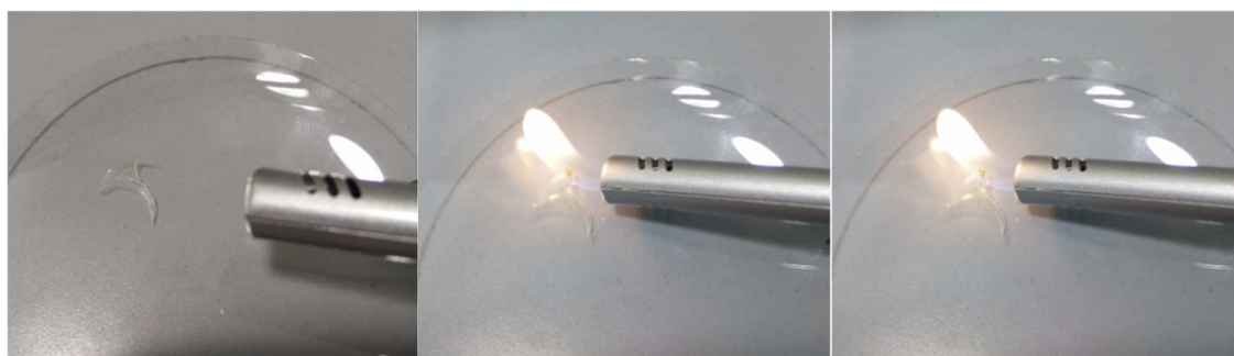
Figure S3. Flammability test of the PEO based polymer electrolytes, incorporating nonflammable IL PyrH4TFSI. Only colour and size changes are visible, no flame originating from the membrane itself.
