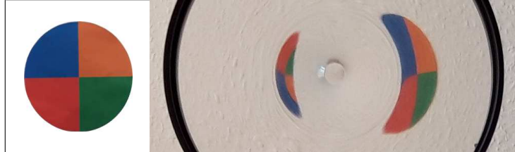
Figure 3.5: Example of parity for images from a lensed source. Left: Original un-lensed source (disk of 6 cm diameter). Right: Images produced when the source is seen through a plexiglass lens that reproduces the lensing effects of a point mass lens. Thanks to the different colours, we can observe that the image on the right (same side as the source) is oriented exactly as the source, thus it has positive parity. The image on the left instead is upside-down, inverted about the horizontal axis, hence the parity is negative. (Picture taken with our own equipment, see section 3.3.2.3)
