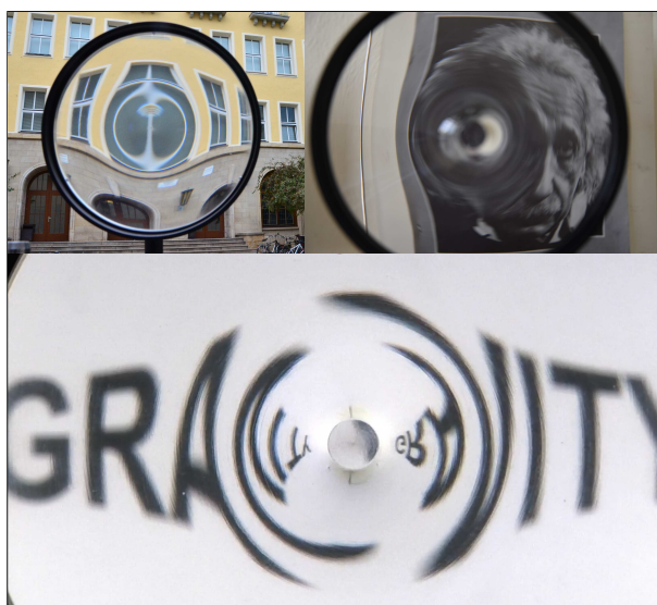
Figure 3.52: Playing with the lenses. Above: Our faculty building through the Plummer sphere lens (left), a portrait of Einstein through the point mass lens (right). Bottom: The word "GRAVITY" through the point mass lens, inspired by [37]. This last picture shows how images seen through the lenses can also be inverted.
