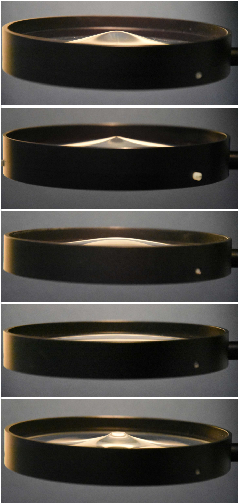
Figure E.2: The five lenses we produced. From left to right: point mass ( R_S = 0.09 cm), uniform disk, Plummer sphere ( R_S = 0.25 cm), SIS and Kuzmin disk ( R_S = 0.25 cm) models.
