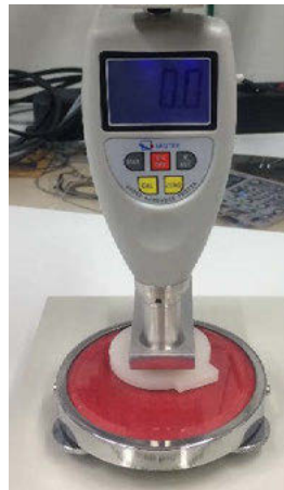
Figure 2: A test sample is placed on the stand hardness tester.
