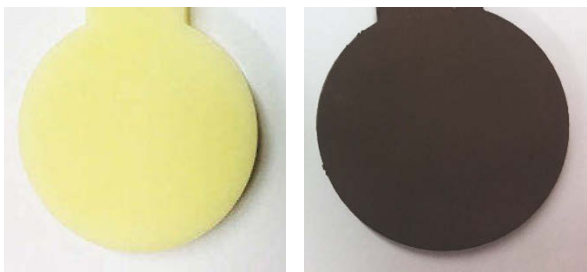
Figure 1: Test samples according to ISO 7619-1:2010 with 6 mm thickness and 5 cm diameter: uncoated sample (left) and Ag/AgCl coated sample (right).
