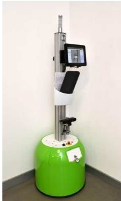
Figure 1. The mobile robotic system based on the MetraLabs Tory platform.
