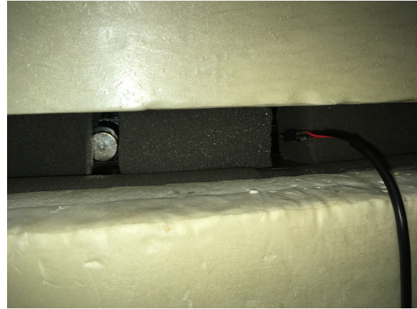
Figure A.4: The insulation at the sidewall with foam material. During the measurements the foam permanently covers the sidewalls except for that, at which the white light sheet enters the cell. At this sidewall the foam material is temporarily removed for the duration of the recording of each image series. Due to the fact, that the temperature in the lab environment is adapted to the average temperature of the working fluid in the cell and the sidewalls are made of glass, this insulation can be considered as an add-on, in order to minimize the heat flux through the sidewalls with regard to the adiabatic boundary condition.
