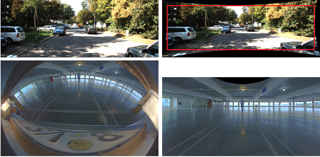
Figure 4.4 Illustration of distortion correction in KITTI and WoodScape datasets.
