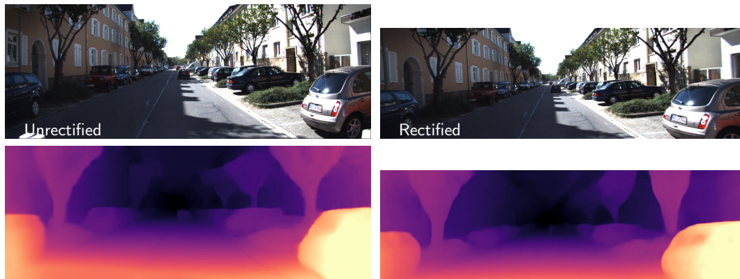
Figure 4.8 Depth obtained from a single unrectified (left) and rectified KITT image (right).
