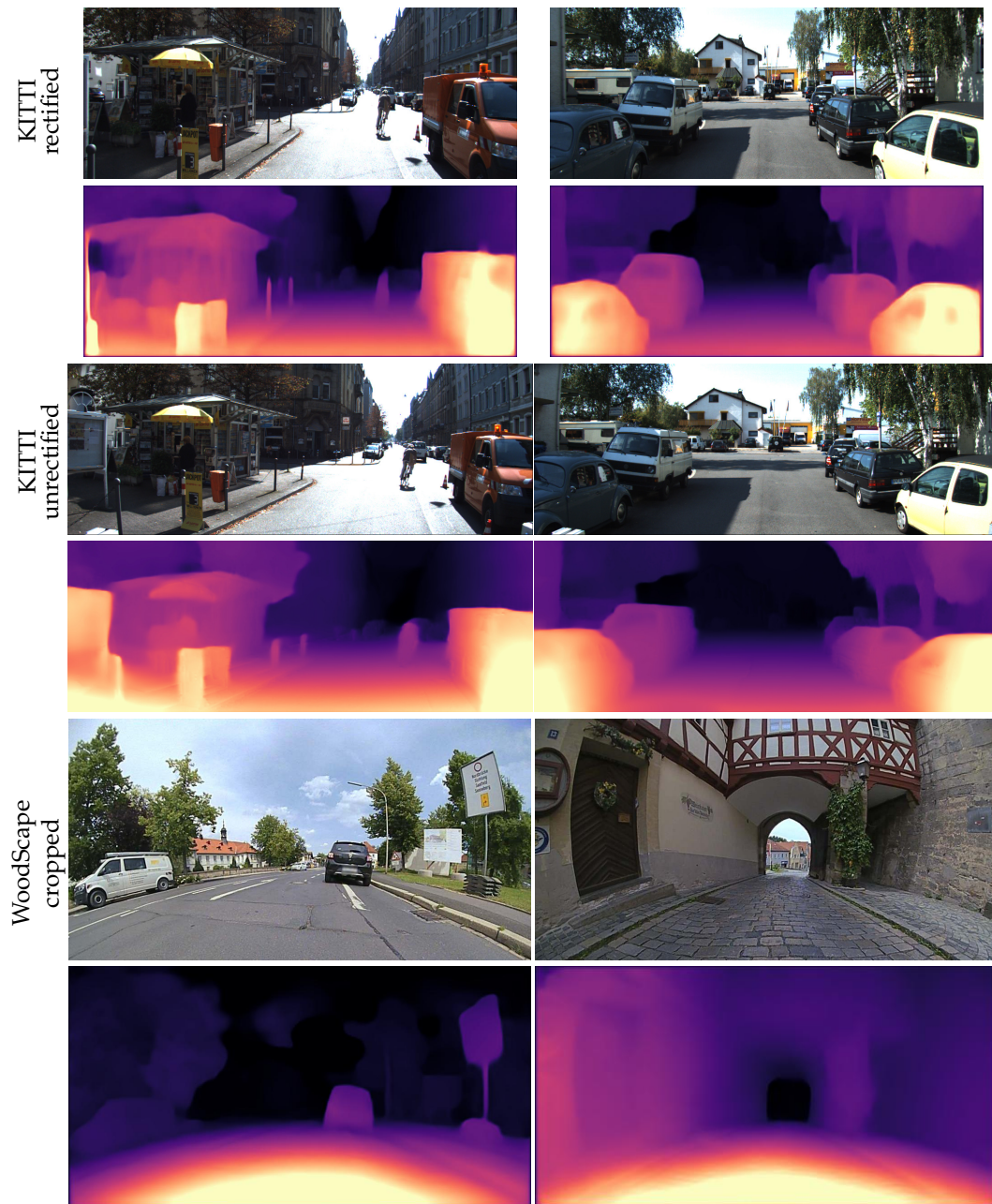
Figure 4.11 Qualitative results comparison of UnRectDepthNet on KITTI and WoodScape dataset. The results on a distorted test video sequence indicate excellent performance, see https://youtu.be/K6pbx3bU4Ss .
