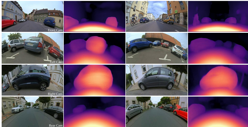
Figure 5.8 Distance estimation results on a surround-view camera system.
