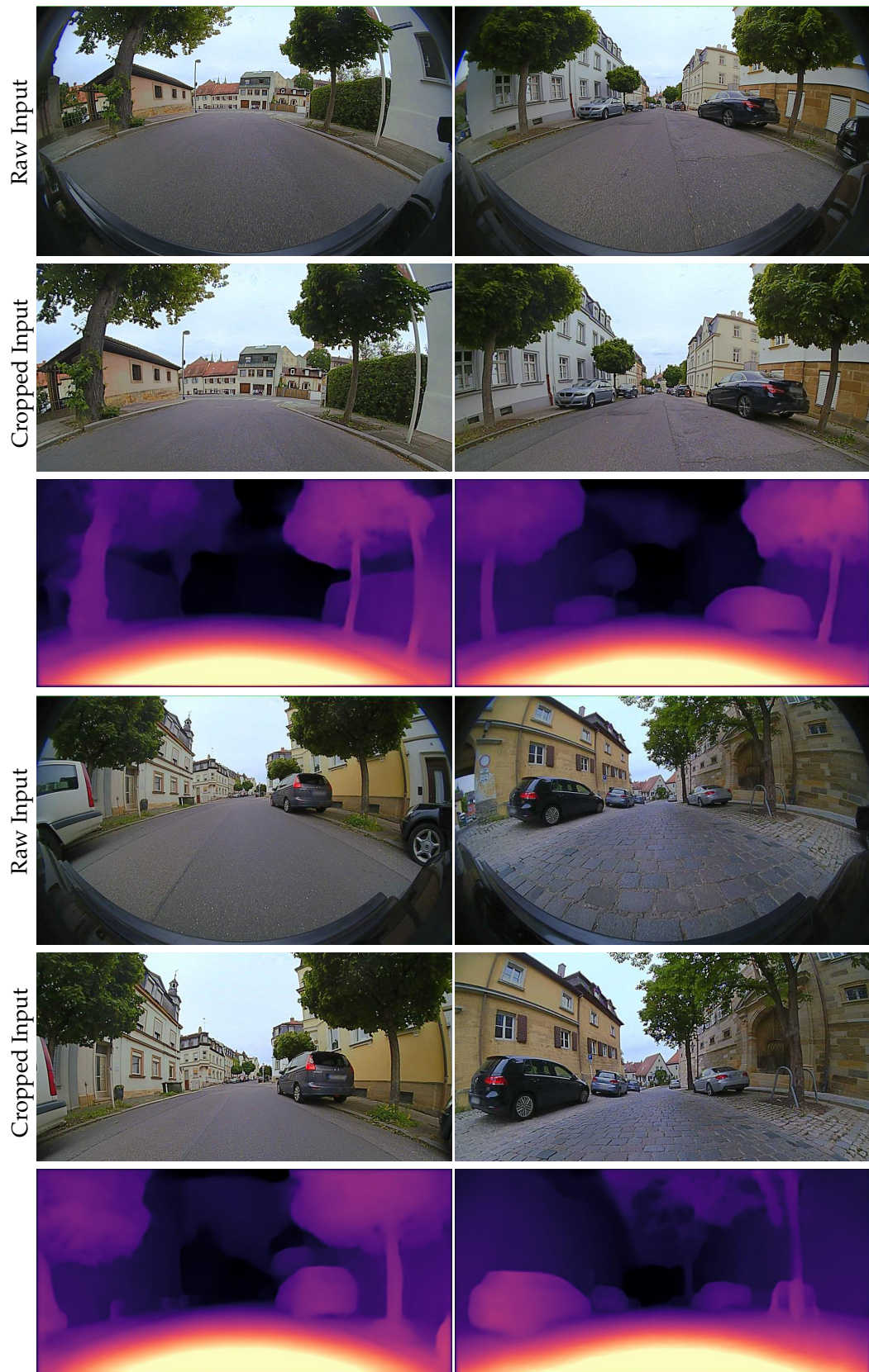
Figure 4.10 Qualitative results of FisheyeDistanceNet on the WoodScape dataset. For more qualitative results, we refer to this video: https://youtu.be/Sgq1WzoOmXg .
