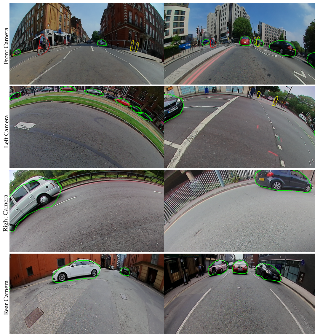
Figure 7.2 Qualitative results of 24-sided polygon-based objection detection on the WoodScape dataset.
