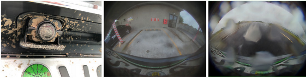
Figure 2.18 Automotive surround-view cameras are exposed to harsh environmental setup. Left: camera lens covered by mud. Middle: image produced by the soiled camera from the left picture. Right: camera lens soiled during heavy rain.
