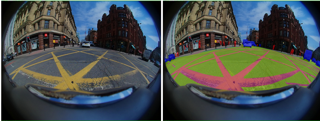
Figure 2.16 A qualitative input sample (left) and semantic segmentation prediction (right) on WoodScape [12].
