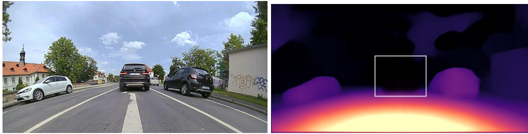
Figure 8.4 Depiction of infinite distance due to dynamic objects on FisheyeDistanceNet inducing holes during inference.
