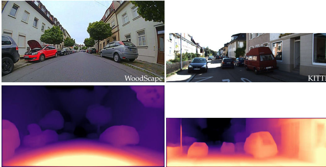
Figure 4.5 Distance and depth derived from a single fisheye image (left) and single pinhole image (right) respectively.
