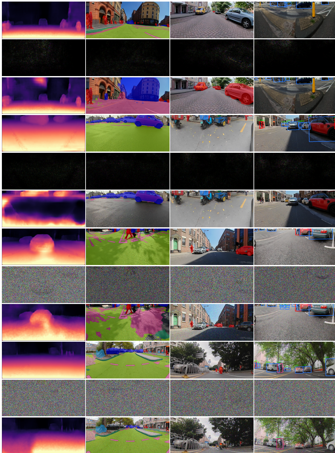
Figure 7.14 From Top to Bottom: White box Untargeted, White box Targeted, Black box Untargeted, and Black box Targeted Attacks. Within each group from top to bottom: Original results, adversarial perturbations, and the impacted results. For intuitive visualizations of the attacks, see https://youtu.be/R3JUV41aiPY .
