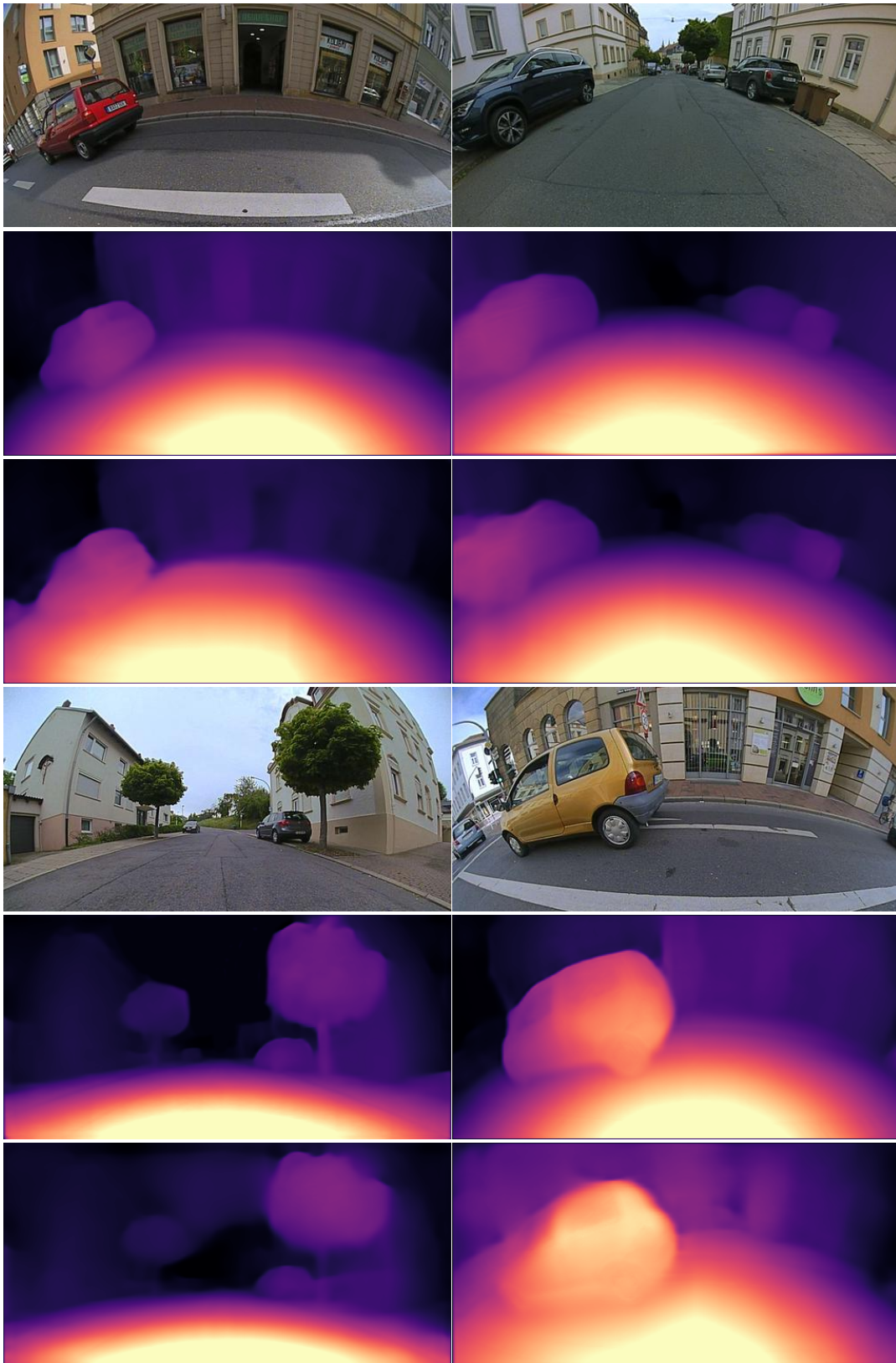
Figure 5.9 Qualitative results of SVDistNet on an unseen sequences from one of the test cars with a different camera intrinsic. The 1 st and 4 th row indicates the raw input images from the front and left camera. The 2 nd , 5 th , 3 rd and 6 th row indicate the distance estimates of the network trained with and without CGT respectively. Despite the notable variation in the camera parameters, the network with CGT outputs sharp distance maps on which edges are visible.
