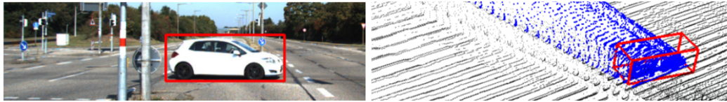
Figure 8.9 Illustration of bleeding edge effect. Figure reproduced from [463].
