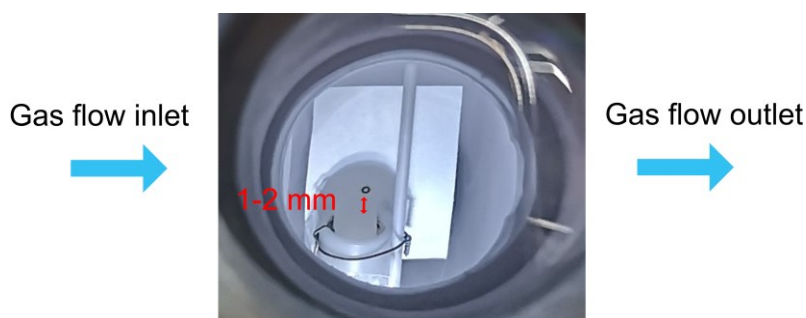
Fig. 4.7 Coal powder or particle holder construction in the gas oven. The view is taken from the laser beam output window. The hole burned into the paper shows the typical probing position.
