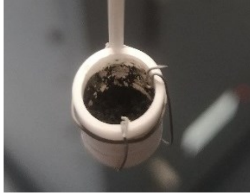
Fig. 7.9 The coal powder state after the gasification measurements implemented at 2.8 bar.
