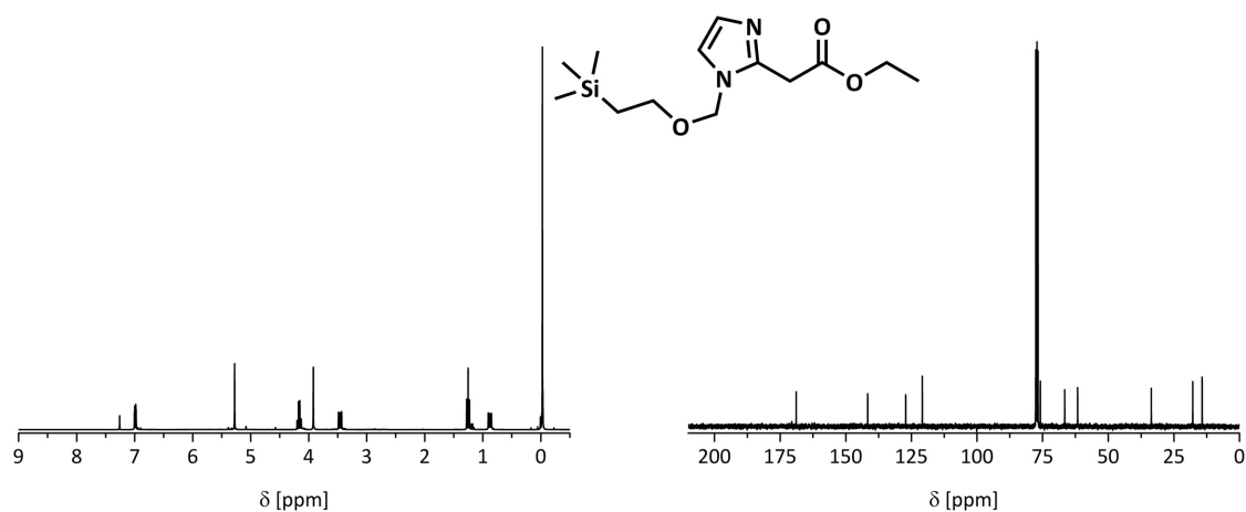
Figure 6.3: 1 H NMR spectrum (left) and 13 C NMR spectrum (right) of 29 in CDCl 3 .
