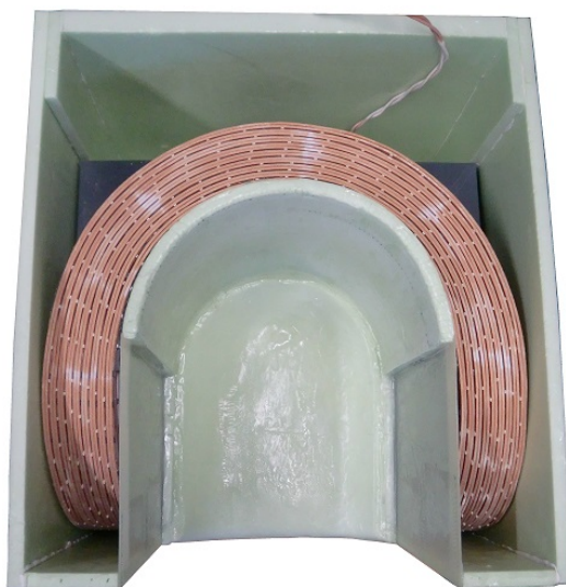
Figure 7.2: Photograph showing a top view of the optimized polarization coil in the oil vessel (oil not inserted).
