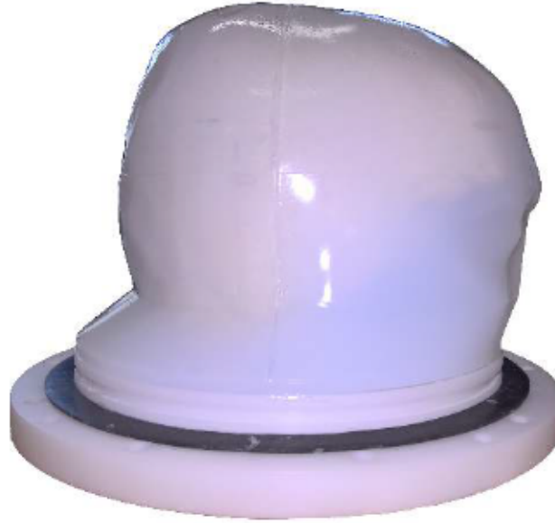
Figure 4.14: Finished phantom in upright position on ground plate with scalp (semi-transparent) on skull (white). The black ring is a sealing used in scalp casting.
