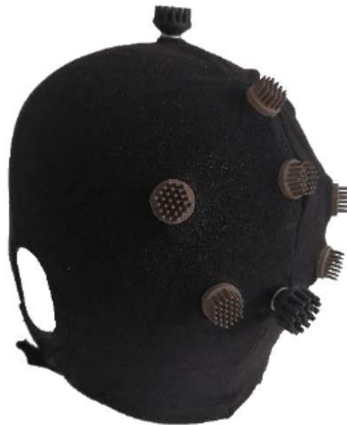
Figure 3.17: The advanced bifunctional cap (black textile) with dry stimulation electrodes printed of eccPLA (black multi-pin electrodes at Cz and Oz) and dry EEG electrodes (grey multi-pin electrodes at Pz, POz, PO3, PO4, O1 and O2). The cap is turned inside out on this photo.
