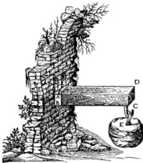
Figure 3: Model of a beam under bending — Galilei, source: http://www.statik-lernen.de/gif/geschichte/galileo_balken.gif
