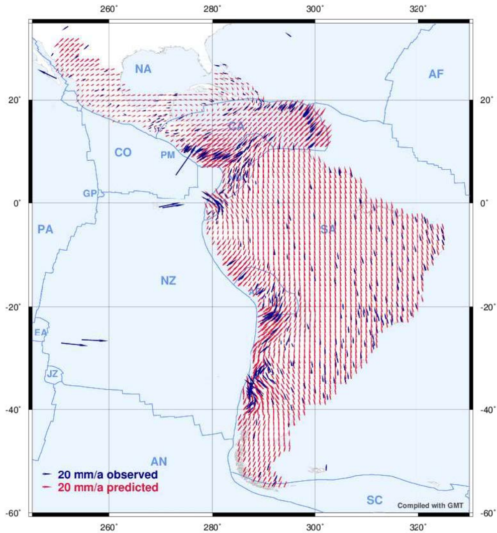
Figure 2.8: Velocity field VEMOS2017 with respect to the South American plate from Drewes and Sanchez (2017).
