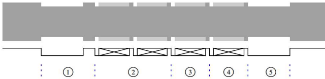
Fig. 4.1 Communication frame from reader to tag of readout includes ①: SOF, ②: Tag ID, ③: Command ID, ④: Memory address and ⑤: EOF.
