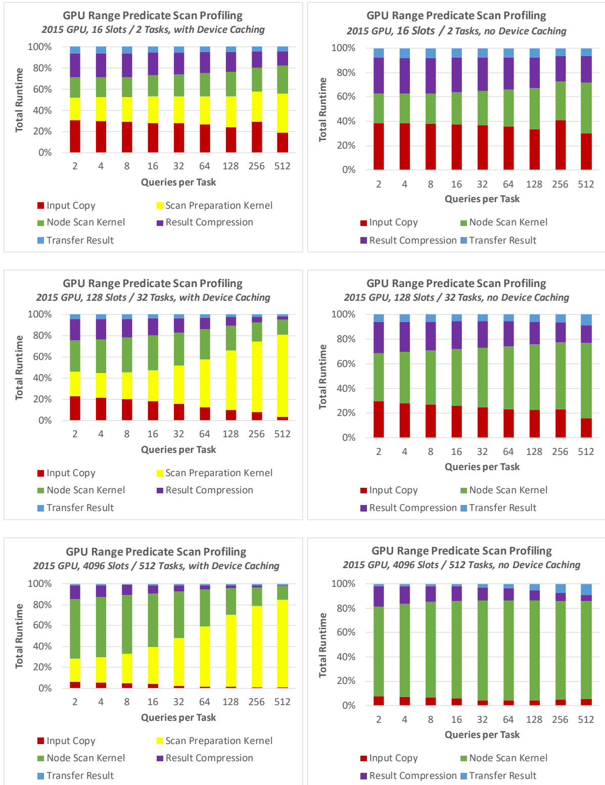
Figure 5.16: Profiling GPU R-Tree Range Predicate Evaluation (2015 Hardware) Low / Medium / High Parallelism Workloads (top / middle / bottom), With / Without on-Device Scan Data Caching (left / right)
