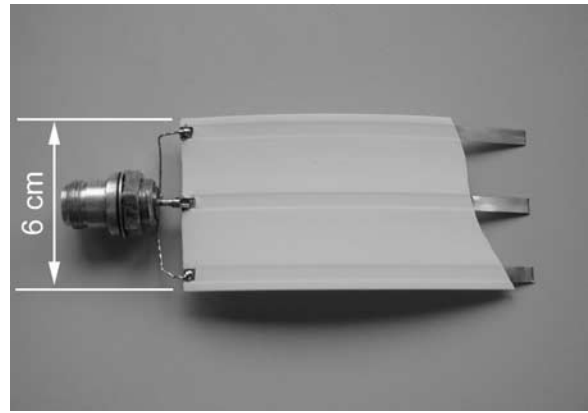
Figure 1. Flat ribbon cable consisting of three copper wires with polyethylene insulation.
