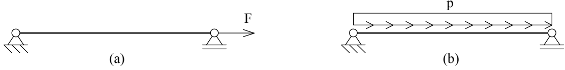
Fig. 5.3: Static systems of a bar problem: (a) a bar loaded by F and (b) bar with constant line load p .
