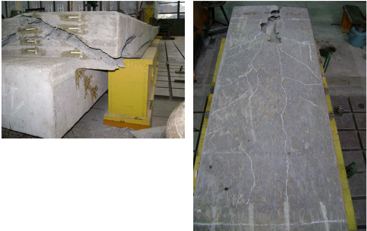
Fig.14 i 15. View of the destroyed element (side and underneath view)
