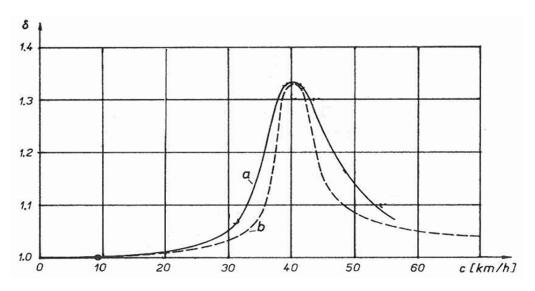
Figure 6: The maximum dynamic deflection in relation to the speed [5], (a) the sprung mass model and (b) the constant load model added to it a harmonic component
