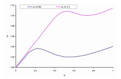
Figure 5: Effect of the ratio between the weights of the vehicle and the beam ( $\kappa$ ) on the maximum dynamic deflection ( $\delta$ ) [5]
