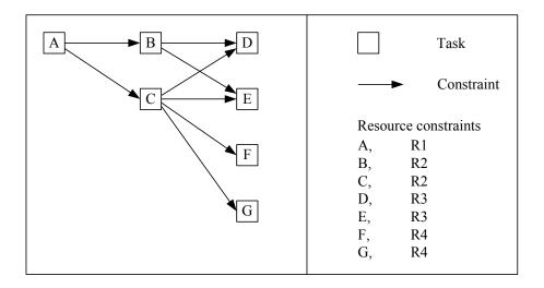
Figure 4: Topological ordering of construction tasks
