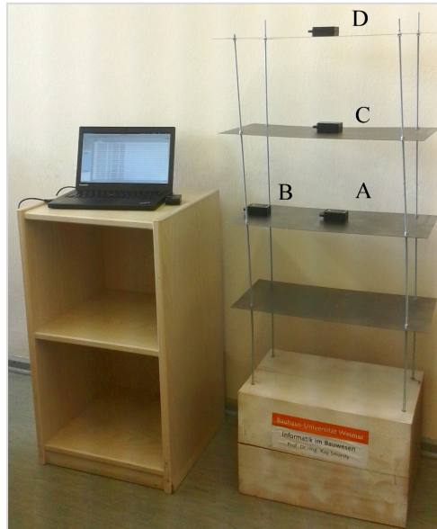
Figure 3: Instrumentation of the test structure
