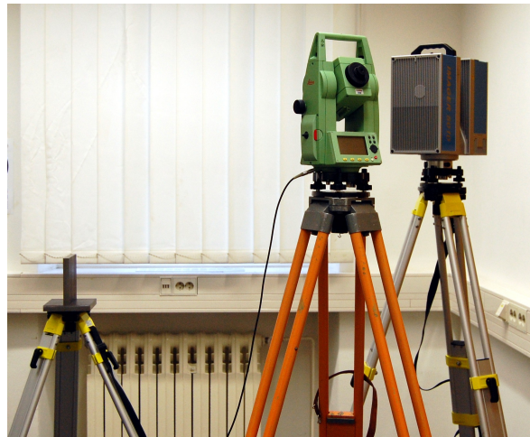
Figure 3: Laboratory setting: T-beam (left), total station (middle) and laser scanner (right)
