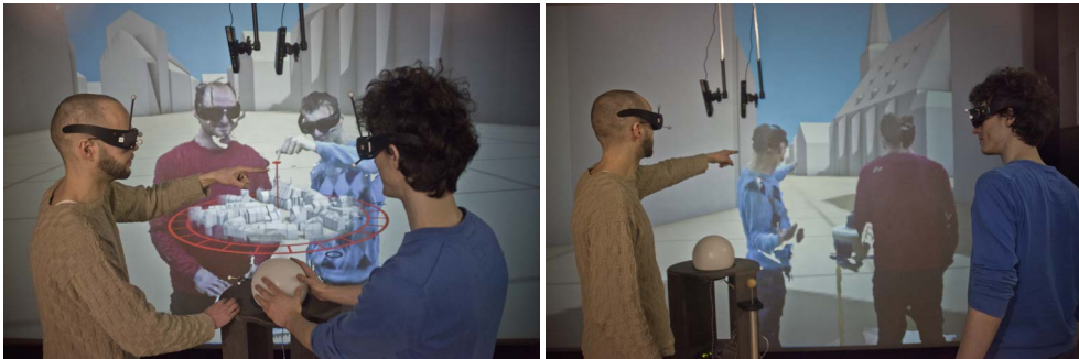
Figure 11.2: Group navigation in a telepresence setting. Left: Two groups use a world in miniature to find their position in the virtual environment. Right: One group follows the other during a virtual city tour. Figures reprinted from [26] © 2013 IEEE
