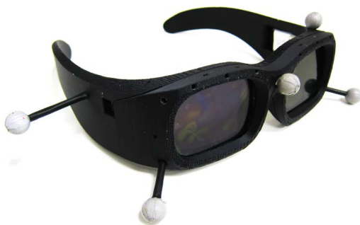
Figure 10.6: Our custom shutter glasses consist of two double cell shutters, a Zigbee radio module, a rechargeable lithium-polymer battery and the shutter driving circuit. The housing also contains multiple threaded holes for assembling different IR-reflective marker configurations.
