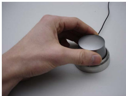
Figure 8.2: The Spacetraveller 3D input device
