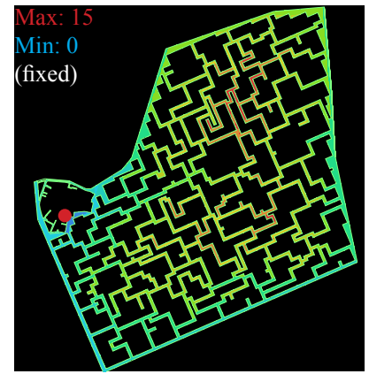
Fig. 20 Step Depth in Random Arrangement
