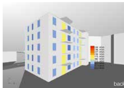
Window dimensions and total radiation entering the windows of the adapted Situation for southern Italy.
