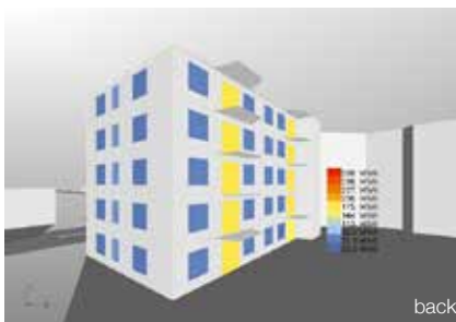
Window dimensions and total radiation entering the windows of the initial Situation for southern Italy.
