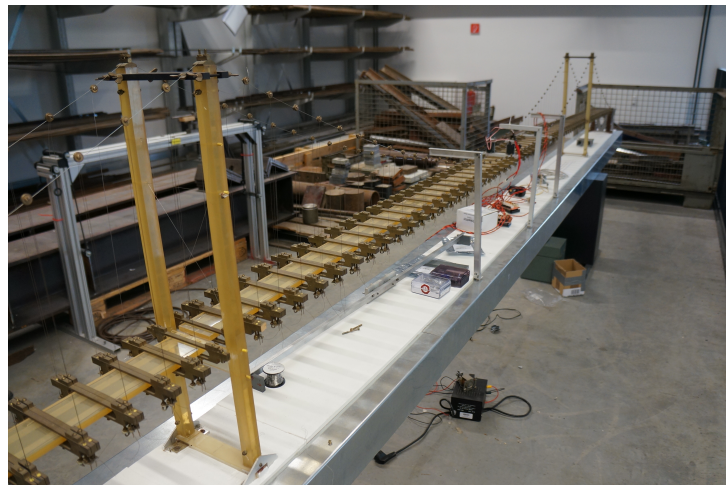
Figure 3: Physical model of the Lillebælt suspension bridge.
