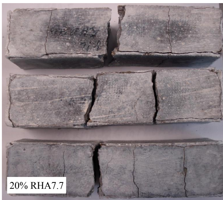
Fig. 9.4 Disruption of the sample containing greywacke and 20 wt.% RHA7.7 in NaOH 1M at 80 °C after 56 days
