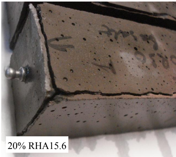
Fig. 9.5 Sample containing 20 wt.% RHA15.6 and basalt aggregate in the NaOH 1M at 80 °C, after 28 days
