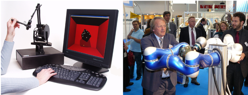
Figure 2.8: The PHANToM force feedback system was the first commercially available system [Web11h] (left), the LWR III of the DLR can be used for two-handed manipulation of virtual objects [HSA + 08] (right).
