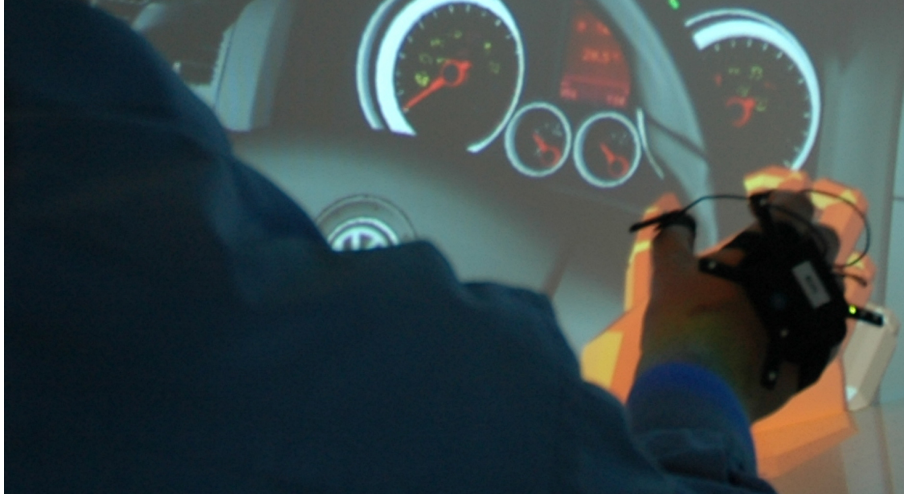
Figure 5.4: Visual feedback in the CAVE, coloring virtual finger segments which are involved in a valid grasp.
