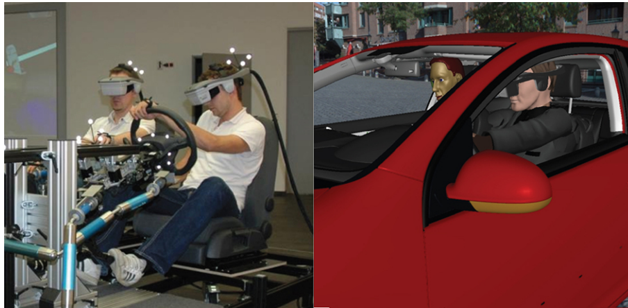
Figure 1.2: A two-user seating buck application for the assessment of electronic car interfaces [SF08]
