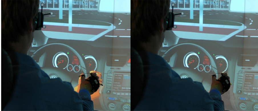
Figure 5.22: The two conditions of the study on the influence of the virtual hand representation on the interaction metaphor: hand condition (left) and no-hand condition (right)
