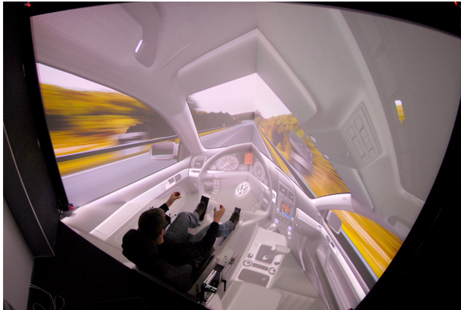
Figure 1.1: Typical CAVE application with a user evaluating a virtual car interior
