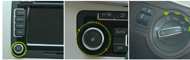
Figure 3.14: Examples for functional constraints: unrestricted controller (left), freely rotatable controller with discrete rotation (middle) and a controller with discrete lock positions and stop positions, the controller cannot be rotated beyond (right)
