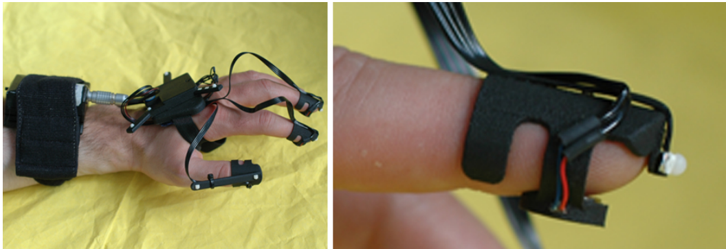
Figure 4.8: Vibration-based feedback device (left) with a close up of the voice coil motor incorporated into the finger thimbles (right)
