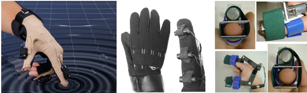
Figure 2.10: The commercially available CyberTouch™ [Web10b] (left), the tactile feedback glove incorporating voice-coil motors introduced by Pabon et al. [PSL + 07] (middle), Inaba and Fujita suggested tactile feedback at the finger tips with a motor driven belt [IF06] (right).
