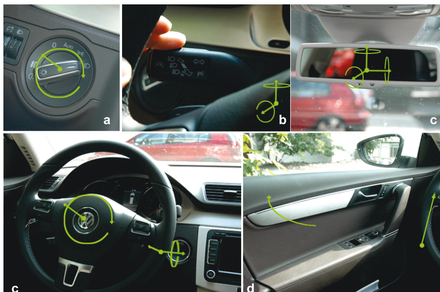
Figure 3.11: Typical mounting constraints found in the car interior: 1R object mounted with a revolute joint (a), a 2R object, mounted with a saddle joint (b), a freely rotateable object, restricted by a ball and socket joint (c), a 1R object additionally movable with respect to a kinematic chain, defined by a 1R hinge joint and a 1T prismatic joint (d) and a 1R object, mounted with a hinge joint (e)
