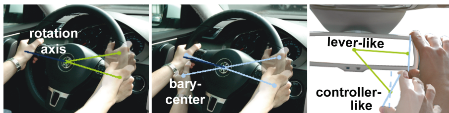
Figure 3.12: Rotation interaction: For big 1R objects both types of rotation — lever-like (left) and controller-like rotation (middle) — have to be provided, for 3R objects a combination of both rotation types results in plausible object motion (right)
