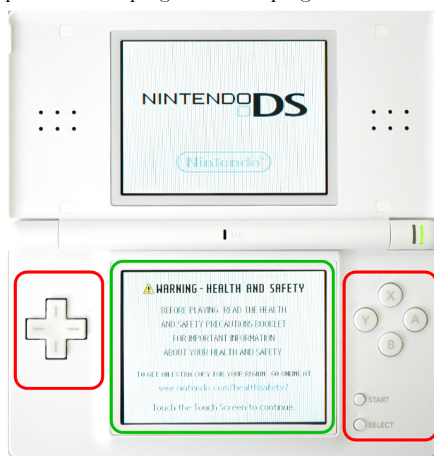
Picture 1: Interface of the Nintendo DS. Besides a conventional interface (red outline) inherited from predecessors like the Nintendo Gameboy, the DS introduced touchscreen interaction (green outline) to mainstream computer gaming source: Wikimedia Commons, Image taken by Havoc
