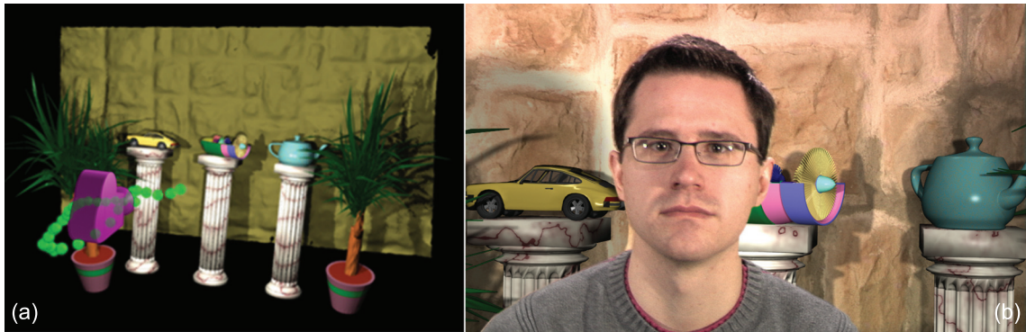
Figure 5.4: Using the projector-camera system to reconstruct the projection surface (a) makes it possible to correctly simulate shadow casts between real and virtual parts of the composite (b).
