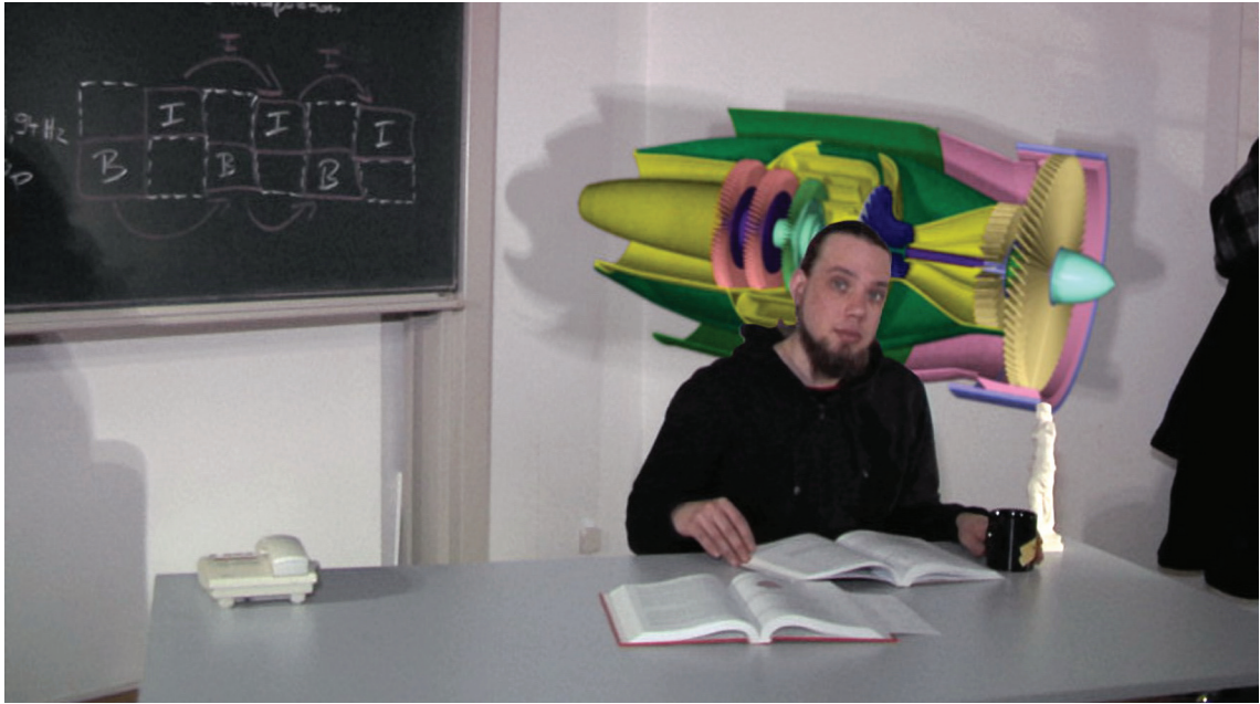
Figure 5.5: Another example composite. Note the shadows which are cast correctly from the augmented turbine onto the real walls.
