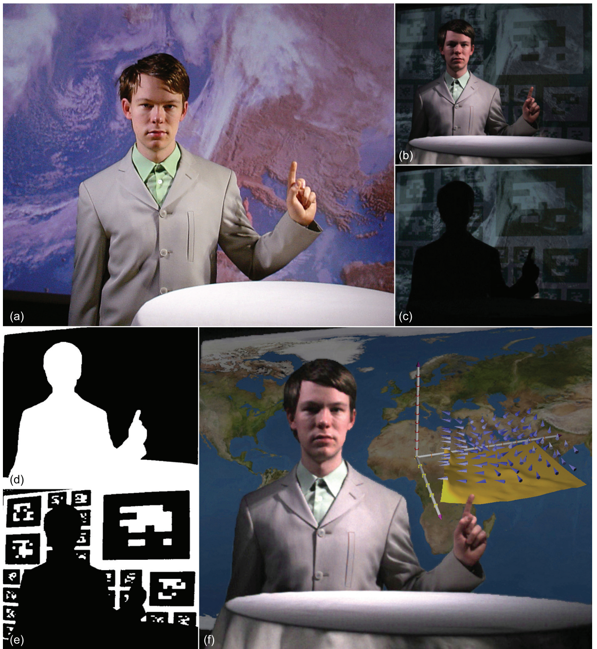
Figure 4.1: A TV studio mock-up with back projection encoding adaptive imperceptible patterns (a), two consecutive images captured by a synchronized camera at 120 Hz (b, c), computed foreground matte from real-time flash keying (d), extracted multi-resolution marker pattern for in-shot camera pose estimation (e), and composite frame with virtual background and 3D augmentation (f).
