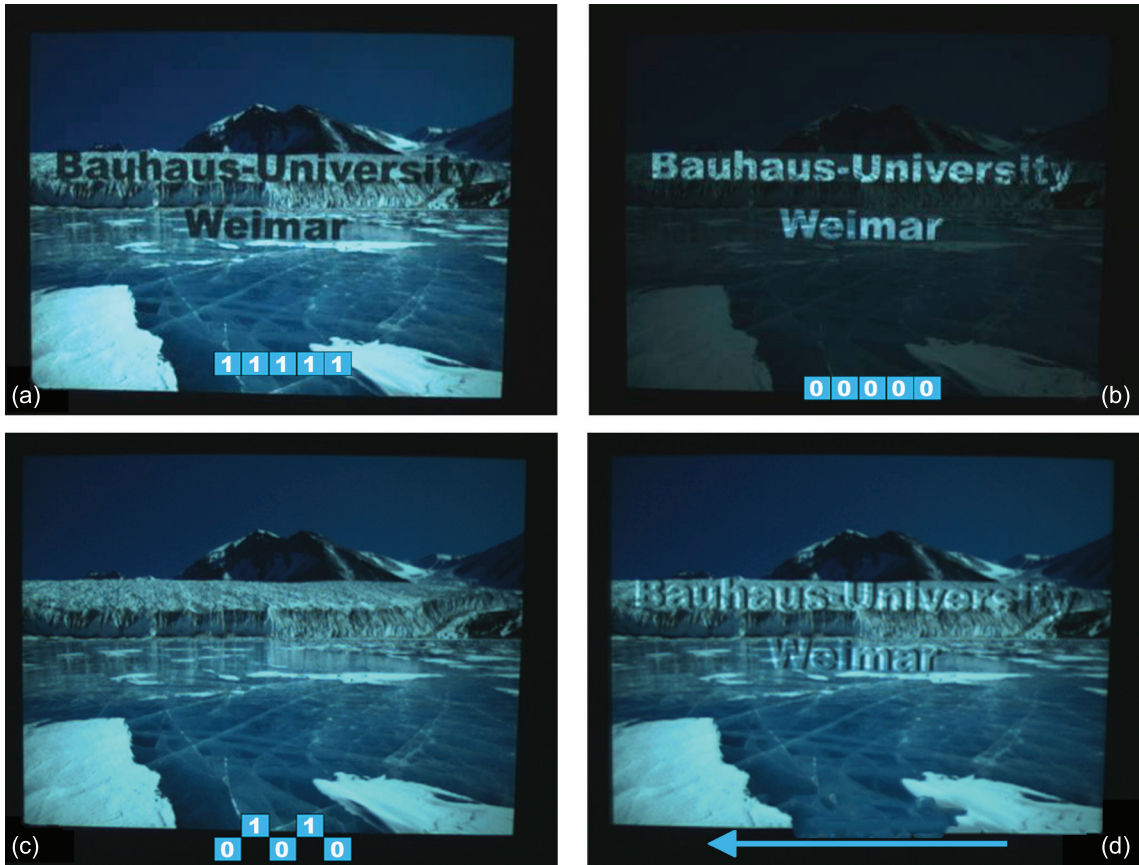
Figure 4.4: The \Delta -coded image pair (a+b) is projected alternately which leads to a perceived image (c) for no or slow eye movements (the blue squares illustrate the sequence of projected code image and compensation image). During faster eye movements, however, the code becomes temporarily visible (d). Note that the intensity of \Delta is increased in this example for illustration purposes.
