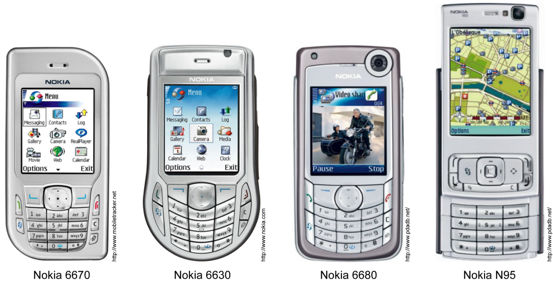
Figure 3.4: The phones used for evaluating the different approaches: Nokia 6670 (CPU: TI OMAP 1510 123MHz; display: 2.1", 176x208; camera: 1.0 MPixel; Bluetooth 1.1, released: October 2004). Nokia 6630, Nokia 6680 (both, CPU: TI OMAP 1710 220MHz; display: 2.1", 176x208; camera: 1.3 MPixel; Bluetooth 1.1, released: November 2004, May 2005). Nokia N95 (CPU: TI OMAP 2420 332 MHz; display: 2.6", 240x320; camera: 5.0 MPixel; Bluetooth 2.0, released: March 2007) [49].
