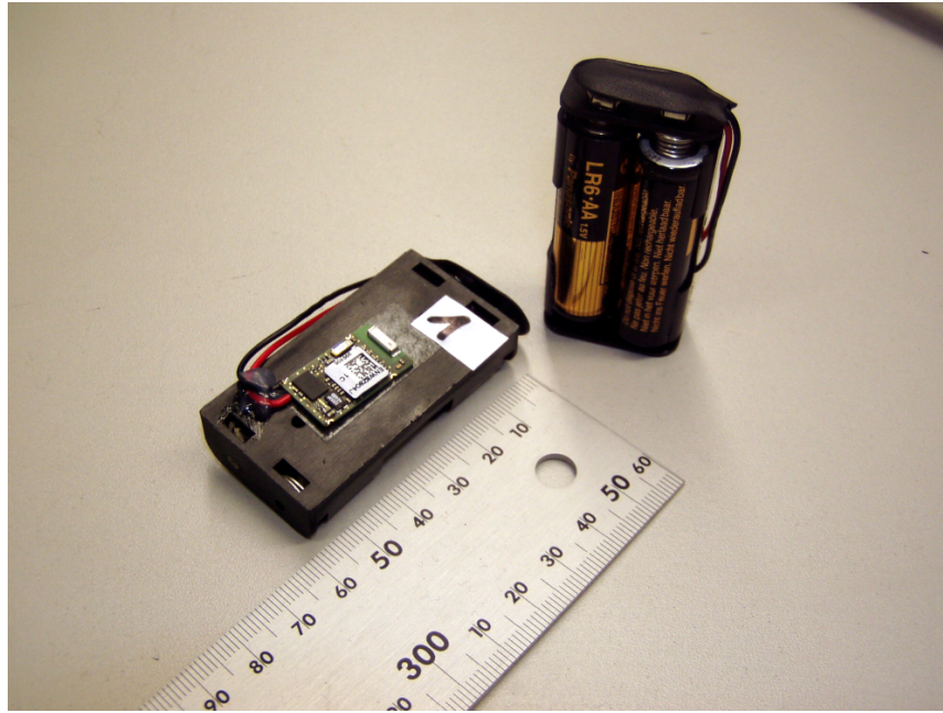
Figure 3.3: Bluetooth emitter [175] with battery pack (scale in millimeter). The Bluetooth beacons are distributed throughout the museum to ensure cell-based localization.
