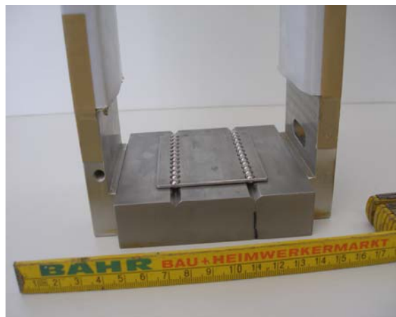
Figure (4.15) Side platens: (a) plane view and cross section; (b) photograph of the side platens covered with Teflon sheets; and (c) close view of the ball bearing
