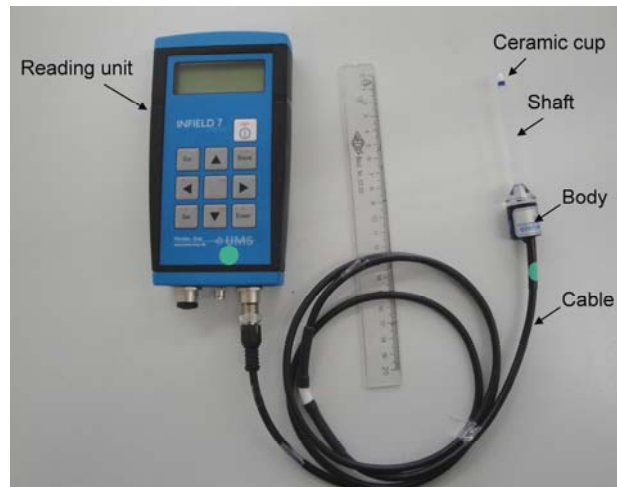
Figure (4.48) Photograph of the tensiometer (type T5) and the reading unit
