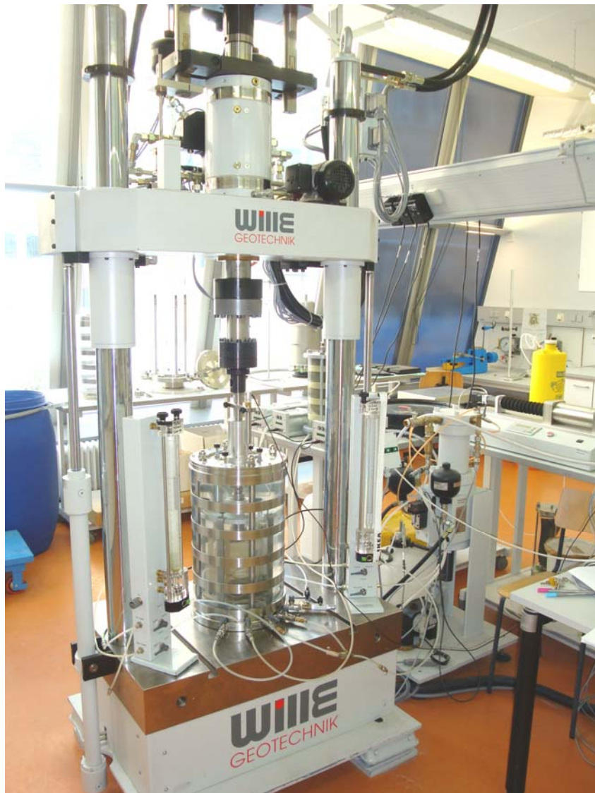
Figure (4.8) Biaxial test set up: the cell is seated in loading frame
