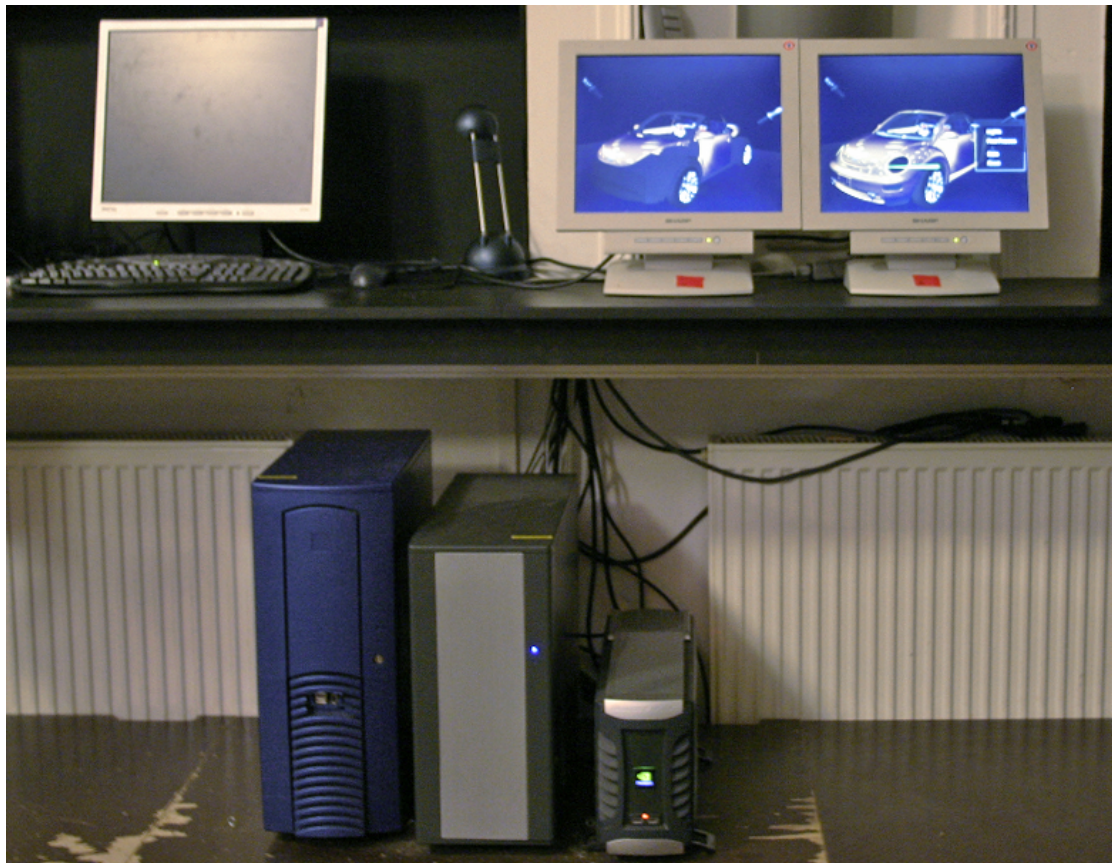
Figure 5.3: Multi-GPU Hardware Setup. PC in the middle is the render client. The graphics sub-system, smaller box right beside the render PC, is provided by an NVIDIA Quadro Plex (cf. figure 5.4) with four outputs: two for the passive-stereo projection system (fast client output) and two for the output devices in the upper right corner of the image (slow client output). In the image the output displays in the upper right show the slow client's left eye image on the left monitor and the fast client's left eye image on the right monitor for demonstration purposes.
