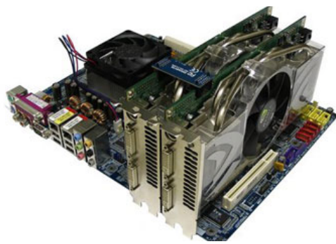
(a) NVIDIA SLI using 2 \times NVIDIA GeForce 8800.
