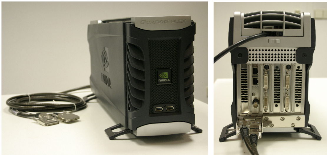
Figure 5.4: NVIDIA Quadro Plex using 2 × NVIDIA Quadro FX 5600 plus NVIDIA G-Sync (second slot from the left in the rear view).
