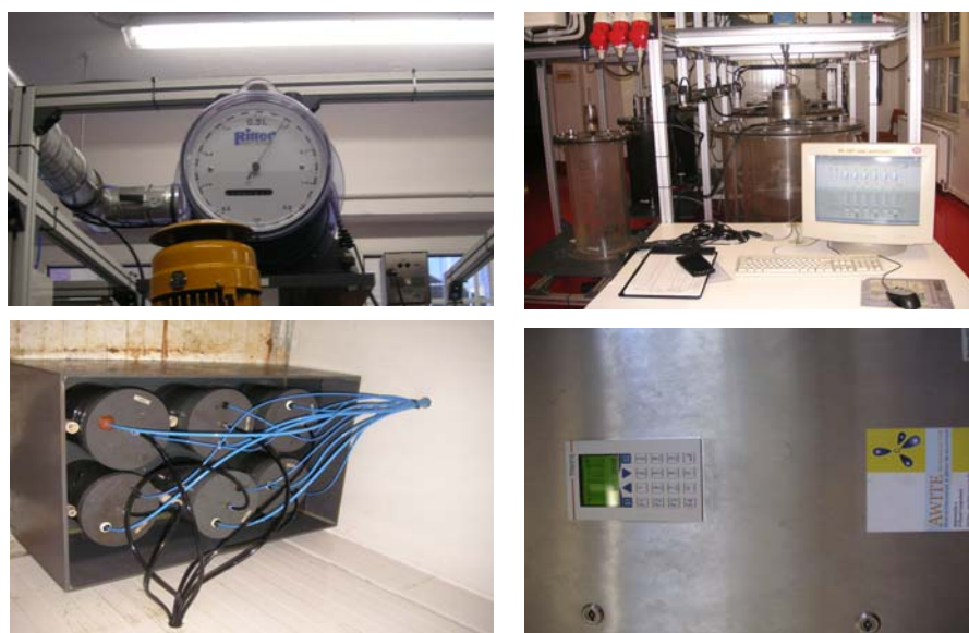
Fig. 5.5: Apparatus for the measuring, storage and analysis of gas
