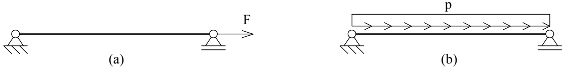
Figure 4.4: Static systems of a bar problem: (a) a bar loaded by F and (b) bar with constant line load p .
