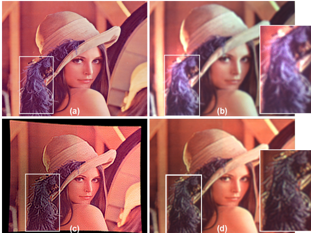
Figure 3. The presentation of an image (a) with a defocused projector (b) can be enhanced by our compensation approach that implicitly sharpens the compensation image (c) that, projected onto the scene, results in a visually more focused projection (d).
