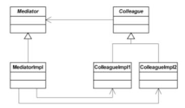
Figure 6. An UML diagram of the mediator design pattern.
