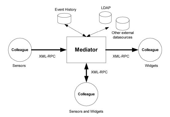
Figure 7. An instantiation of the CORBA mediator pattern.
