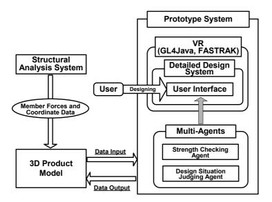
Fig. 3 The developed design environment
