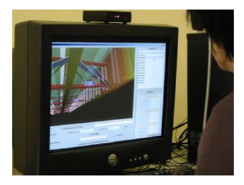
Fig. 6 A selected element of the design member is highlighted by changing its color from yellow to orange
