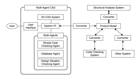
Fig. 1 The previously developed Multi-Agent CAD environment
