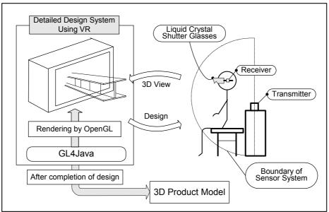
Fig. 4 Detailed design system using virtual reality
