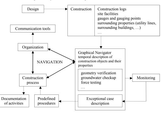
Figure 6: Flow of information in co-operation platform
