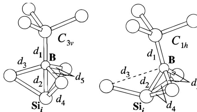
FIG. 6. Atomic structure of the  $A_{Si}-Si_i$  defect for the case of boron in the two possible configuration  $C_{3v}$  and  $C_{1h}$ . (after Ref. 41)
