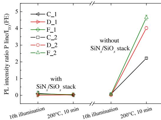
FIG. 4. P line intensity ratio after illumination and annealing with and without protective  $\text{SiN}_x\text{:H/SiO}_x$  stack on the surface of the samples.
