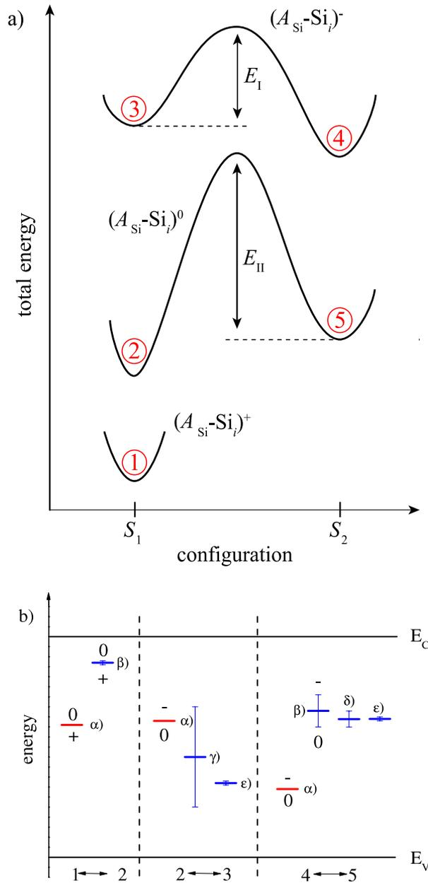
FIG. 7. a) Schematic diagram of total energy curves as function of configuration coordinates for charge states (+), (0) and (-) of the  $A_{Si}-Si_i$  defect in *p*-type silicon. b) Energy diagram of the electronic levels within the bandgap of silicon in the case of the  $B_{Si}-Si_i$  defect. Simulation and measurement data are colored red and blue, respectively. Refs.  $\alpha$ ) 41,  $\beta$ ) 43,  $\gamma$ ) 31,  $\delta$ ) 44,  $\epsilon$ ) 45.
