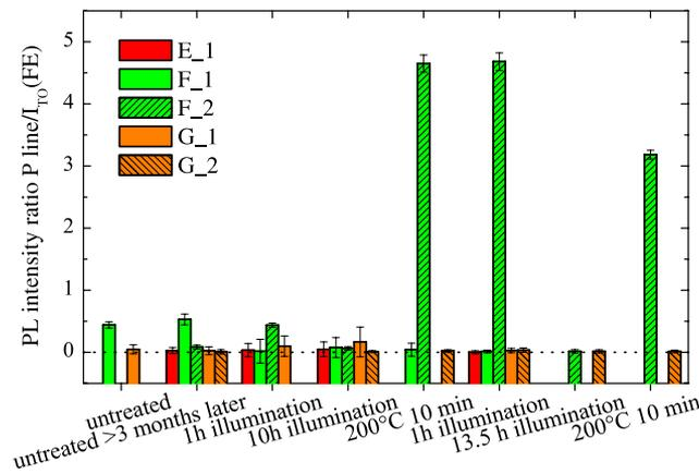
FIG. 3. PL intensity ratio of P line and free exciton during the illumination and annealing treatment for samples implanted with the low indium dose. In the case of missing bars the samples were annealed or illuminated but no measurement was done.
