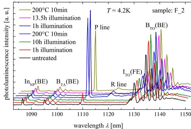
FIG. 2. PL spectra of sample F\_2 after different steps of the illumination and annealing cycle. The spectra are shifted in x and y direction for clarity. The spectra are normalised with respect to the peak height of the free exciton  $I_{TO}(FE)$  peak.
