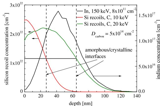
FIG. 1. Simulated concentration profiles of indium and recoiled silicon atoms for both carbon implantation energies (wafer F and G in Tab. I) as a function of depth. The amorphous/crystalline interfaces for each carbon implantation are marked by dashed lines.
