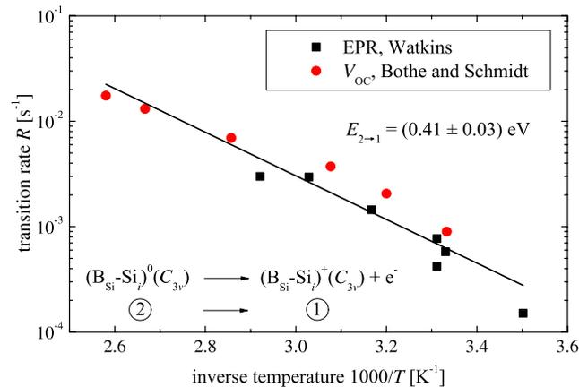
FIG. 8. Arrhenius plot of the transition rate of the  $A_{Si-Si_i}$  defect in case of boron from state 2 to 1 in Fig. 7(a). Data are taken from Refs. 48 and 31
