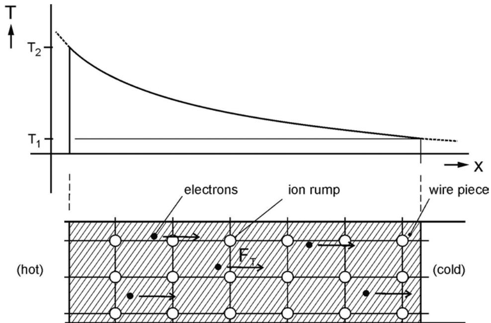
Fig.1 Generalized temperature gradient and electron diffusion in a metallic wire
