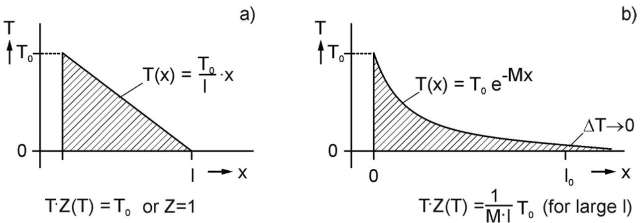
Fig.7 Linear versus exponential drop in temperature over the wire length  $T_0$  maximal temperature.
