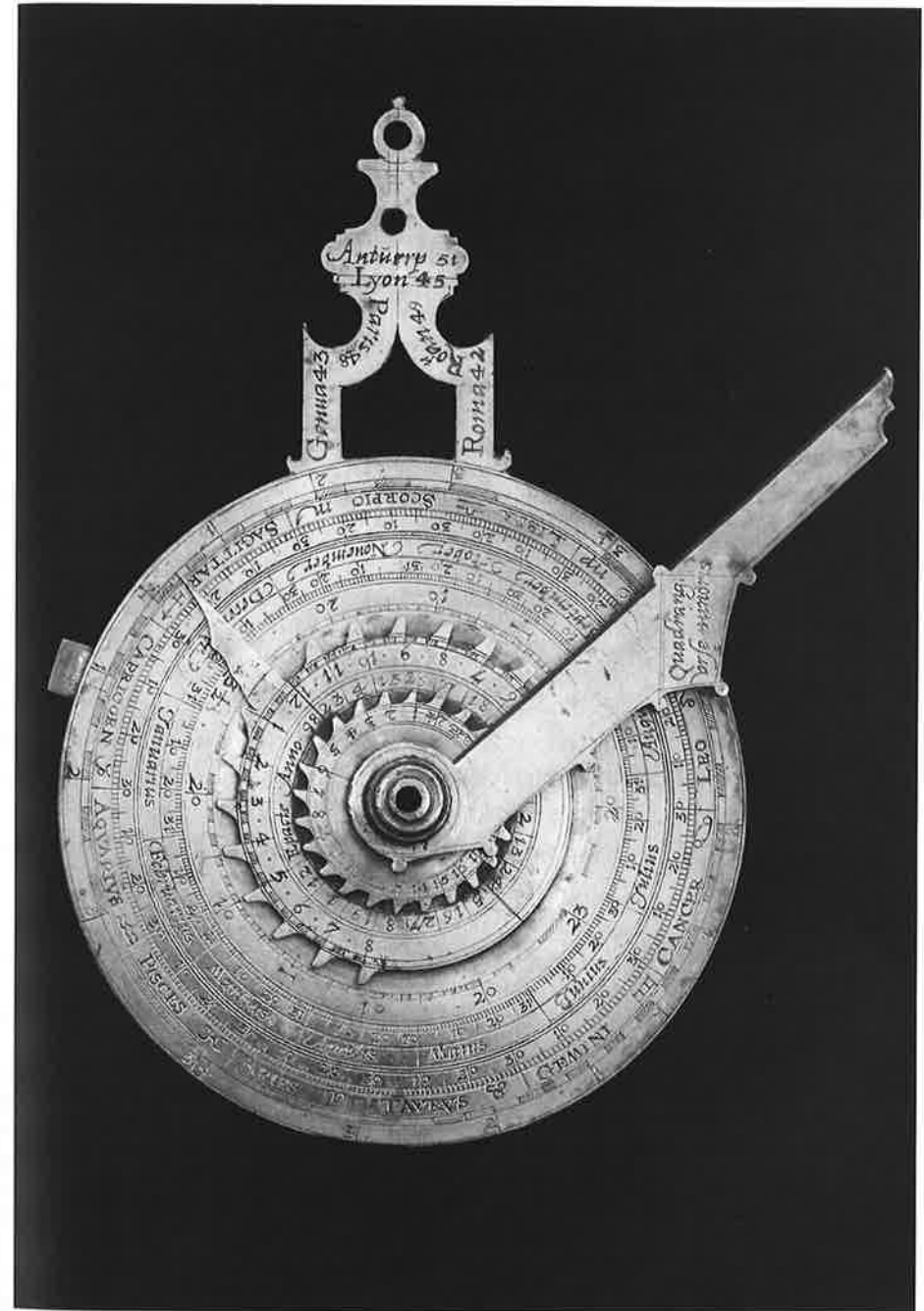
Figure 3: Michiel Coignet, Nocturnal and sundial , 1598 [brass, diameter 108 mm]. (Museum of the History of Science, University of Oxford, inv. 44721)
