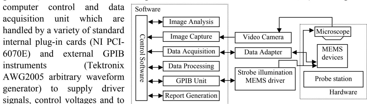
Fig. 1. Diagram of in-plan micro-motions measurement system
