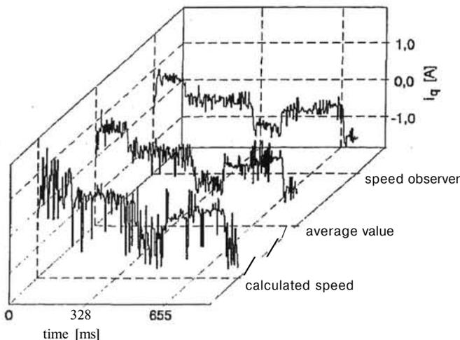
Figure 14: force producing component  $i_q$  during positioning operation
