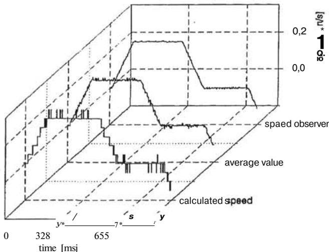
Figure 13: speed during positioning operation
