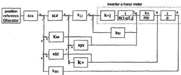
Figure 8: Structure of the complete cascaded state control
