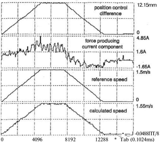
Figure 6: Positioning operation with a speed of 1.5 m/s
