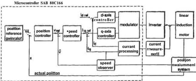
Figure 2: Structure of the cascaded position control
