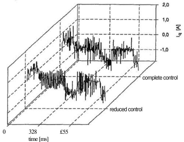
Figure 11: Force producing current component during positioning operation
