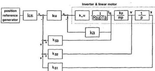
Figure 9: Structure of the reduced state control
