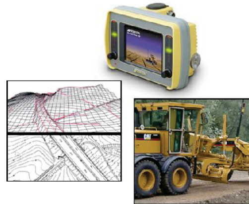
Fig.9: Control and reporting of “As Build” data by on side GPS / WLAN technology (source: TOPCON, RIB AG)
