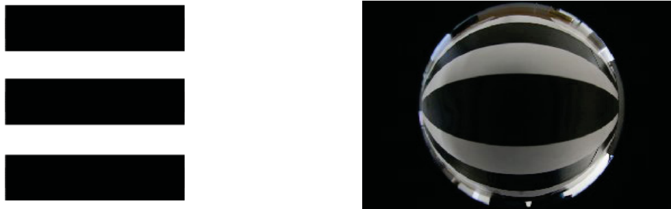
Fig. 2: Image target for the intrinsic camera parameter calibration. A parallel black and white pattern is prepared as a target (left) and is captured through the fish-eye camera which is to be calibrated (right).
