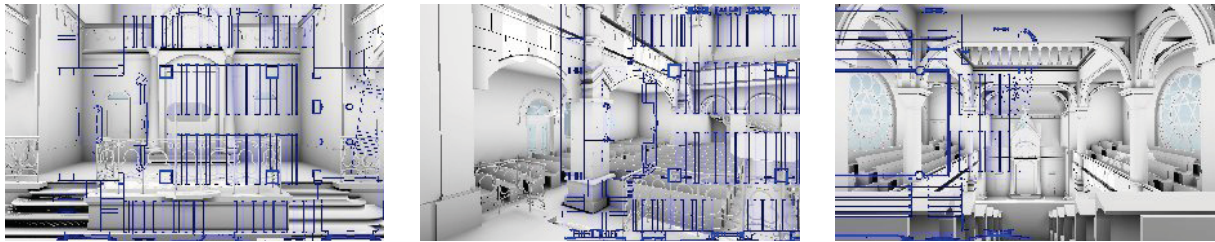
Fig. 5: Superimposition of 3D view and the floor plan showing the user's current position.
