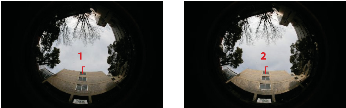
Fig. 11: Captured image pair #1: The camera heights are 0.69m (left) and 0.81 m (right).
