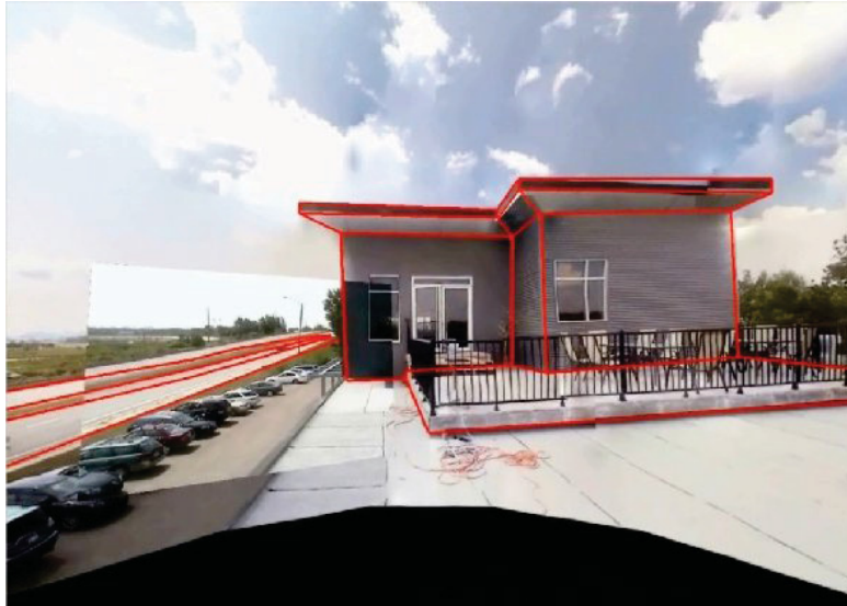
Fig. 3: 3D building model overlaid onto live video, both overlaid onto panorama.
