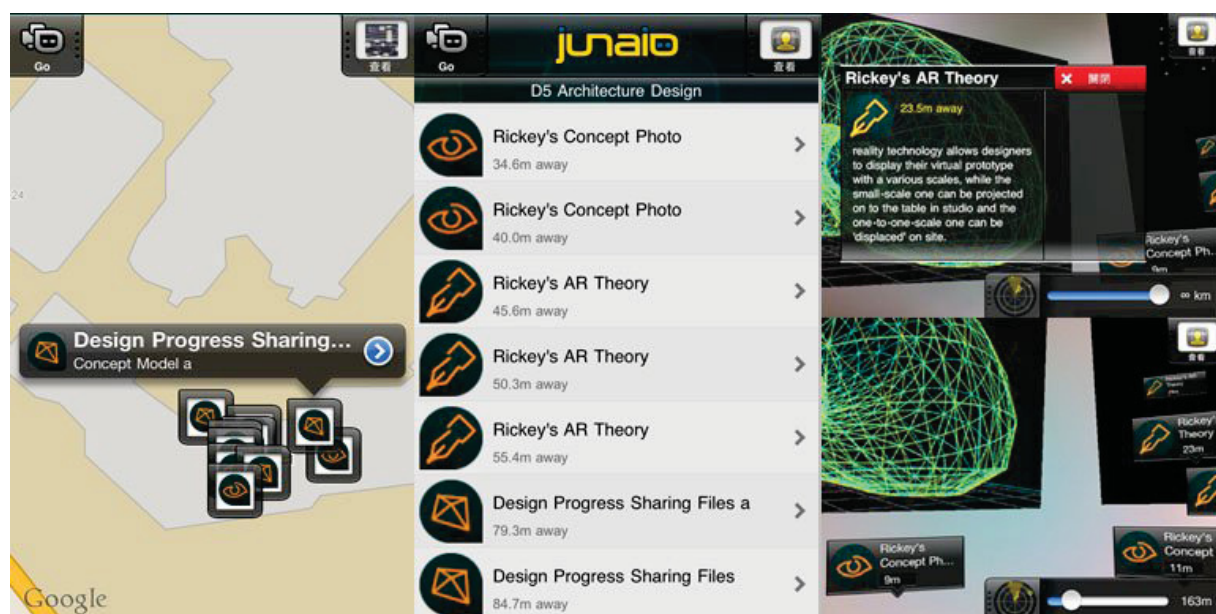
Fig. 6: Three views of informational AR scaffolding, viewed on a map (left), as a list (centre) or in a 'live' spatial view (right), which responds to panning, tilting and movements of the phone. Project by Rickey Gong Wang.
