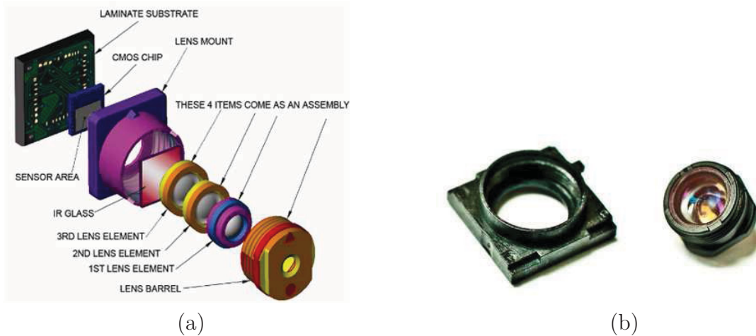
Figure 2.1: (a) Components of a state of the art miniature camera showing a number of plastic molded lenses which are integrated inside a barrel. This is screwed into the lens mount which is subsequently attached to the printed circuit board (PCB, laminate substrate) with bonded CMOS image sensor. An IR cut-off filter glass is included in the lens mount [42]. (b) Photograph of plastic lens barrel and mount [42].
